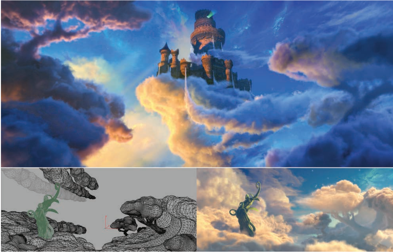
Fig. 1. Top: Shot from the animated feature Puss in Boots , showing high-resolution animated clouds generated using VDB [Miller et al. 2012]. Left: The clouds are initially modelled as polygonal surfaces, then scan-converted into narrow-band level sets, after which procedural noise is applied to create the puffy volumetric look. Right: The final animated sparse volumes typically have bounding voxel resolutions of 15,000 \times 900 \times 500 and are rendered using a proprietary renderer that exploits VDB’s hierarchical tree structure. Images are courtesy of DreamWorks Animation .
