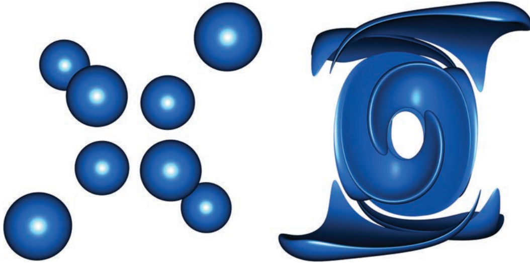
Fig. 10. Left: The “8x” variation of the Enright sphere [Enright et al. 2002], recently introduced in Christensen et al. [2011]. Where the original Enright sphere uses a single sphere of radius 0.15 placed at (0.35, 0.35, 0.35) in a normalized unit box, this “8x” version uses eight spheres with radius 0.125 positioned at (0.35, 0.35, 0.35), (0.15, 0.15, 0.85), (0.15, 0.85, 0.15), (0.35, 0.65, 0.65), (0.85, 0.15, 0.15), (0.65, 0.35, 0.65), (0.65, 0.65, 0.35), and (0.85, 0.85, 0.85). Results are shown for an effective data resolution of 4,096^3 and a narrow-band width of 10, corresponding to 263,418,462 active voxels in the initial level set. Right: Result of divergence-free advection at half-period, where the active voxel count peaks at 1,096,281,344 voxels!
