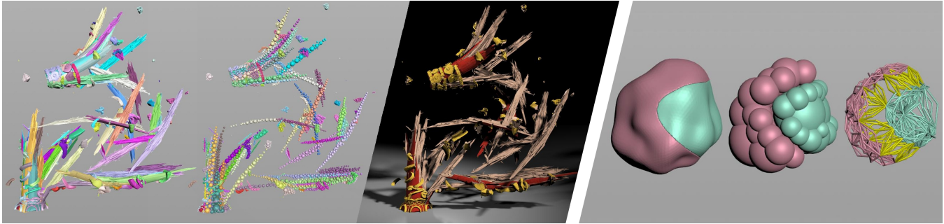
Left: Simulation of a wood column bending & breaking with our system (1.29 sec/frame, 230 fragments, 3.2K bodies, 89K constraints). Right: Volume fracture often results in concave fragments; our decomposition yields no inter-fragment overlap; our custom constraint network.
