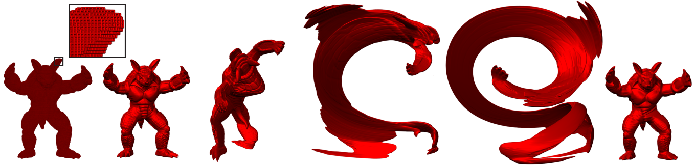
Figure 1: Enright benchmark test on high-resolution DB+Grid. Divergence-free advection of the Armadillo at an effective resolution of 4096^3 . Far-left: Close-up of dynamic 4^3 blocks. Frames show level sets at time= 0, \frac{1}{8}, \frac{1}{4}, \frac{1}{2}, 1 period. Notice how the initial (time= 0 ) and last (time= 1 ) frames appear almost identical, indicating low mass-loss due to numerical dissipation. This is a consequence of the high resolution.
