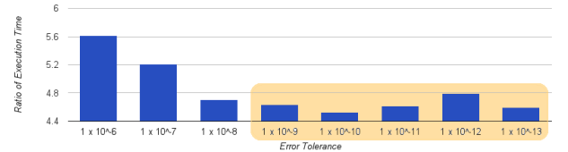
Figure 8: Ratio of execution time for fastCCD to openCCD when processing one million randomly generated collision pairs. With this input data openCCD found 77192 collisions in 8.704 sec. For approximately E_{tol} = 1 \times 10^{-9} or lower, fastCCD produces the same result (shown in the highlighted region). For lower values of the error tolerance, fastCCD reports a small number of additional collisions.
